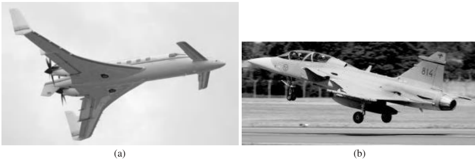
Figure 6.13 Two aircraft with canard configuration: (a) Beech Starship; (b) Saab JAS-39B Gripen. Reproduced from permission of (a) Ken Mist; (b) Antony Osborne.
