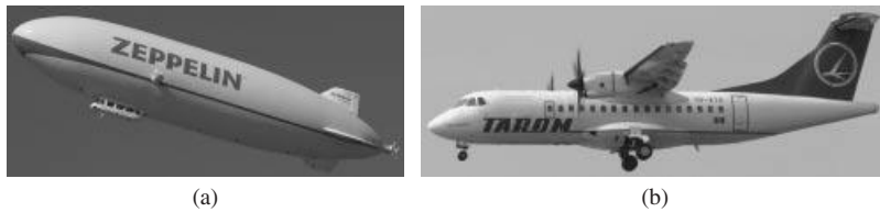
Figure 3.8 Lighter-than-air craft versus heavier-than-air craft: (a) Zeppelin NT; (b) ATR-42. Part (b) reproduced from permission of Anne Deus.
