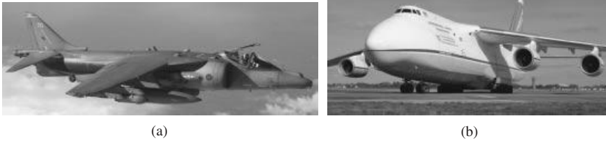
Figure 4.4 (a) British Aerospace Harrier GR9 with a thrust-to-weight ratio of 1.13 and (b) Antonov An-124 with a thrust-to-weight ratio of 0.231. Reproduced from permission of Antony Osborne
