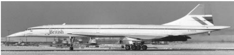
Figure 7.24 Aerospatiale-British Aerospace Concorde with fuselage length-to-diameter ratio 23. Reproduced from permission of A J Best
