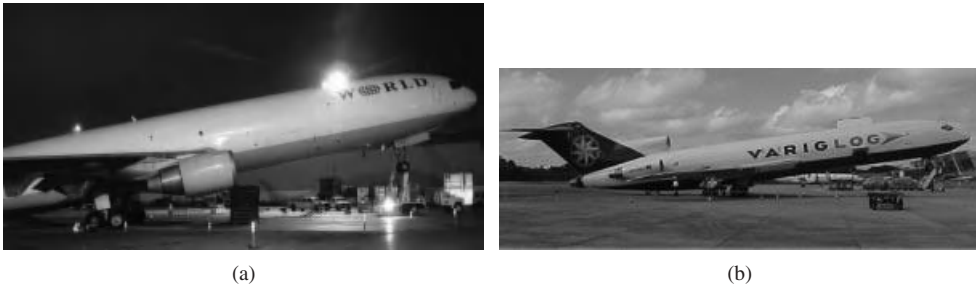
Figure 11.1 Too much load beyond the allowed aft cg creates an accident. (a) A McDonnell Douglas MD-11 nose up due to the cg aft of main gear; (b) A Boeing 727 nose up due to loading error in Brazil, June 9, 2001. Reproduced from permission of (a) Randy Crew; (b) Orlando J. Junior
