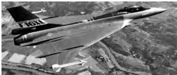
Figure 5.61 Example of a stall fence: (a) Fence over the wing; (b) Fence over the wing of General Dynamics F-16XL
