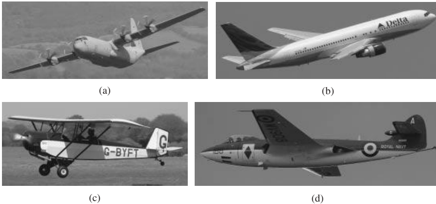
Figure 5.4 Four aircraft with different wing vertical positions: (a) cargo aircraft Lockheed Martin C-130J Hercules (high wing); (b) passenger aircraft Boeing 767 (low wing); (c) home-built aircraft Pietenpol Air Camper-2 (parasol wing); (d) military aircraft Hawker Sea Hawk (mid-wing) (Reproduced from permission of (a, d) Antony Osborne; (b) Anne Deus; (c) Jenny Coffey.)
